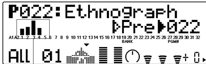
The “level meter” bars indicate the “level” (velocity) of the incoming MIDI data.
