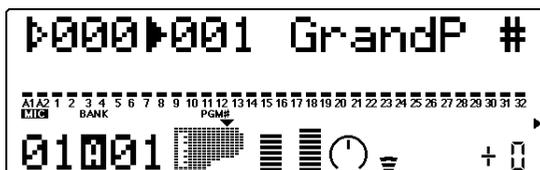
This displays all Parts, but the level meters are at half the height.
