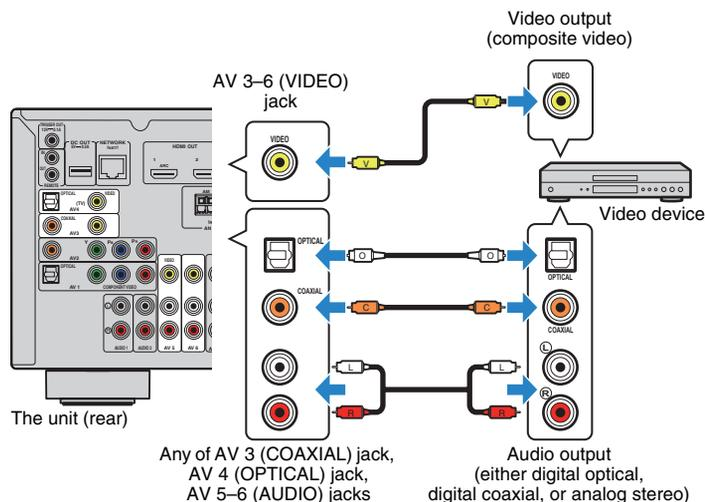
If you select the input source by pressing AV 3-6, the video/audio played back on the video device will be output from the unit.
