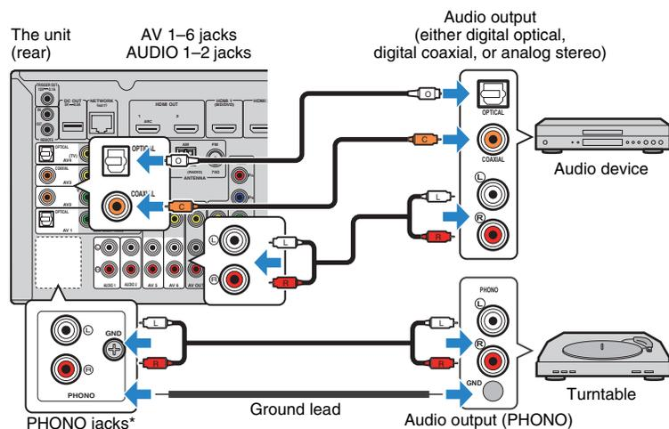
If you select the input source by pressing AV 1-6, AUDIO 1-2 or PHONO\*, the audio played back on the audio device will be output from the unit.
