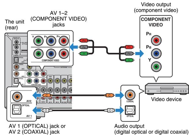
If you select the input source by pressing AV 1-2, the video/audio played back on the video device will be output from the unit.
