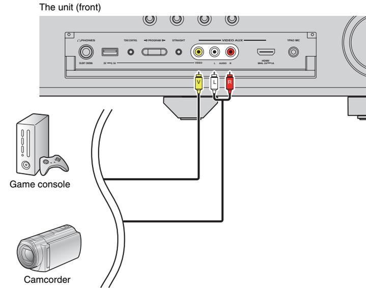
If you select “V-AUX” as the input source by pressing V-AUX, the video/audio played back on the device will be output from the unit.
