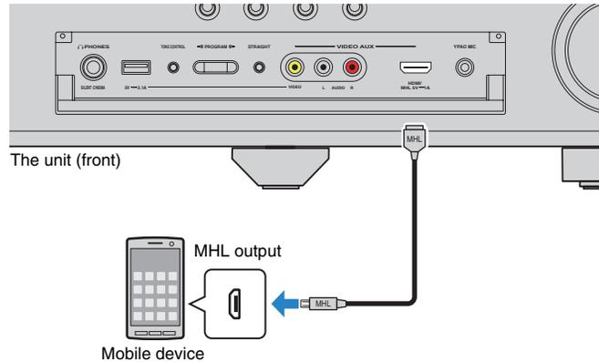
If you select “V-AUX” as the input source by pressing V-AUX, the video/audio played back on the mobile device will be output from the unit.
