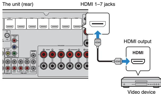
If you select the input source by pressing HDMI 1-7, the video/audio played back on the video device will be output from the unit.
