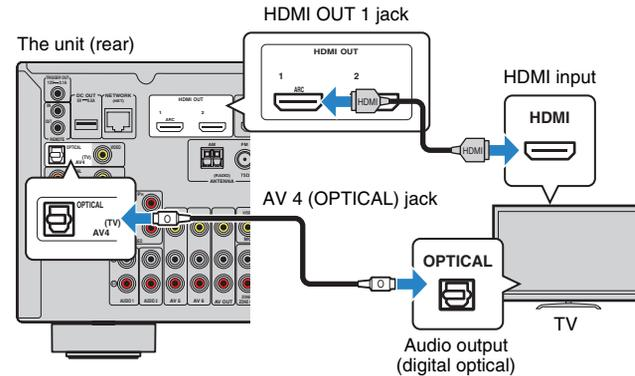
If you switch the input source of the unit to "AV 4" using the AV 4 or SCENE(TV) keys, the TV audio will be played back on the unit.
