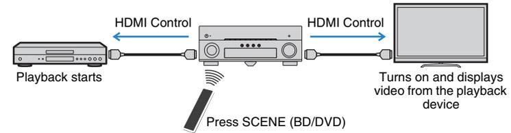
To use HDMI Control, you need to perform the following HDMI Control link setup after connecting the TV and playback devices.
