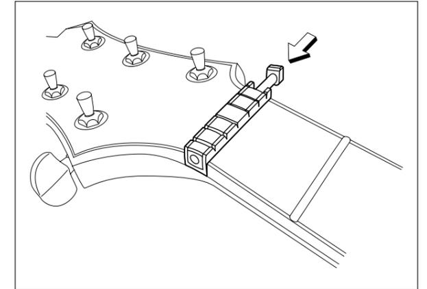
**6** Re-attach the locking lever and tighten lightly.
