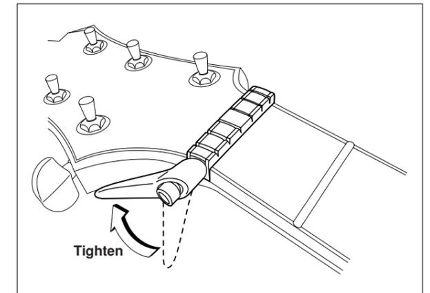
**7** This completes locking block replacement. Install the new strings and tune the guitar. (Refer to the "Installing the new strings" section in the FC Tremolo System Manual.)
