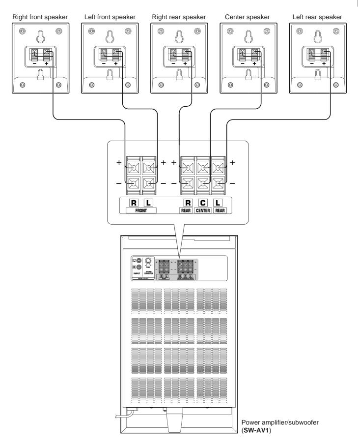
Connect the provided speakers (NX-AV1) to the SPEAKERS terminals on the rear of SW-AV1.
