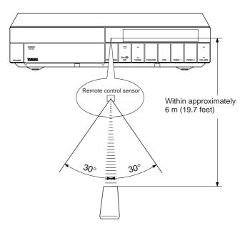
Aim (within the range of 60° with no obstacles) the remote control transmitter at the remote control sensor and operate as shown.
