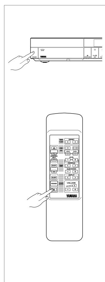
If the AC supply lead is connected to the AC outlet, this system can be turned on and turned into the standby mode by pressing the **POWER** switch on the front panel of the main control unit or the **POWER** switch on the remote control transmitter.
