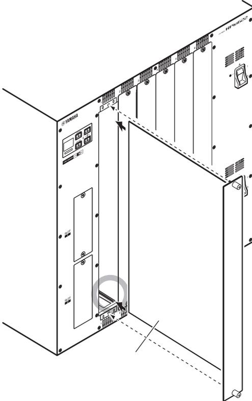
**4** Fasten the card using the screws attached to the card.
