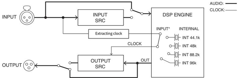
The input SRC converts the signal to the system clock of the RIVAGE PM series. The output SRC converts the signal to the specified internal clock source or to the same clock as the input of the same channel.
