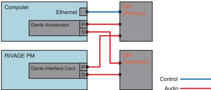
**Connection example when controlling NUENDO Live from the NETWORK [PC] terminal of the SP engine**
