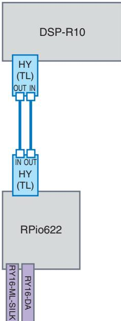
Use fiber-optic cables to connect the TWINLANE IN/OUT jacks of the HY card (installed in the DSP engine) to the TWINLANE OUT/IN jacks of the HY card (installed in the I/O rack).
