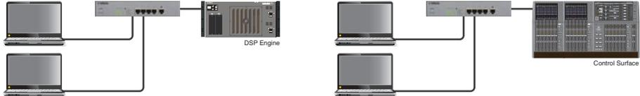
If you want to connect two computers to a DSP engine or control surface, use a switching hub to make connections.
