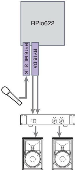
1 Analog input connection Connect a microphone or line-level component to the input jacks of the RY card (RY16-ML-SILK).
