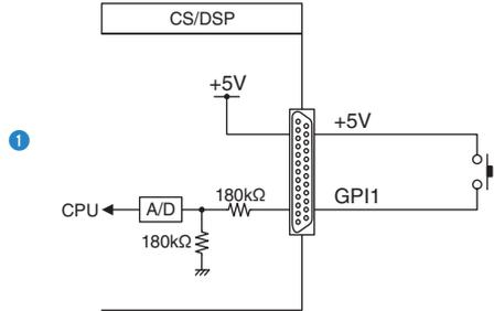
**Using a switch connected to GPI IN8**
