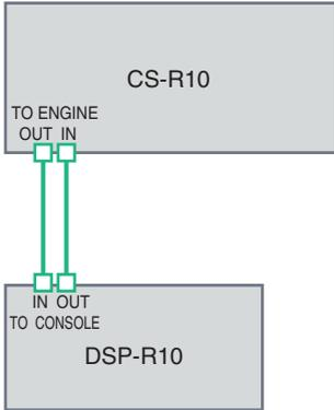
Use Ethernet cables to connect the TO ENGINE OUT/IN jacks of the control surface to the TO CONSOLE OUT/IN jacks of the DSP engine.
