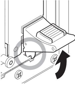
**5 Affix the card using the screws that were previously used to affix the slot cover.**
