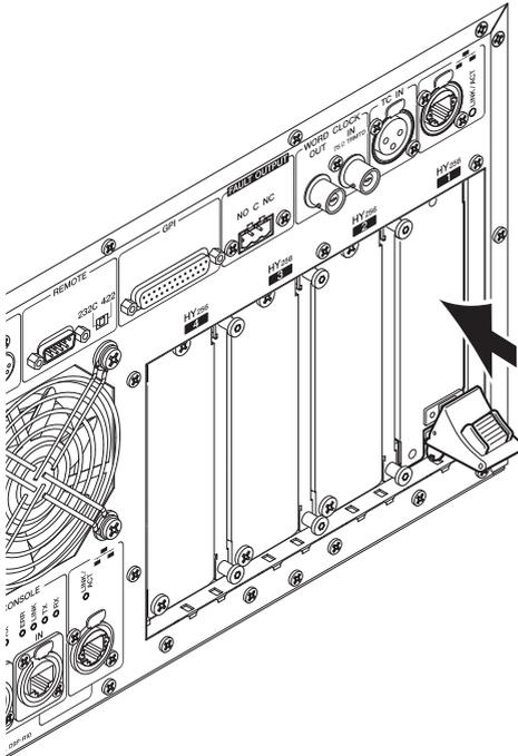
**4 Pull up the card installation lever to lock in the card.**
