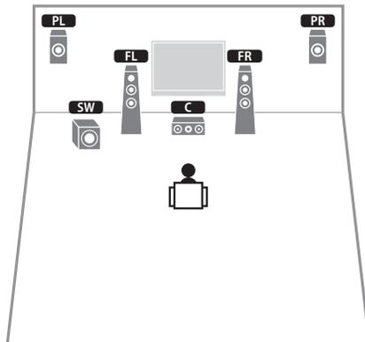
This speaker system uses the front presence speakers to produce a natural 3-dimensional sound field, and creates the virtual surround speakers using the front speakers to allow you to enjoy multi-channel surround sound (Virtual CINEMA DSP).
