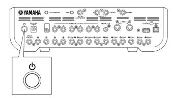
2 Connect the DC plug of the included AC power adaptor to the DC IN jack on the rear panel. To prevent the cord from being unplugged accidentally, wrap the cord around the cable clip and secure it.
