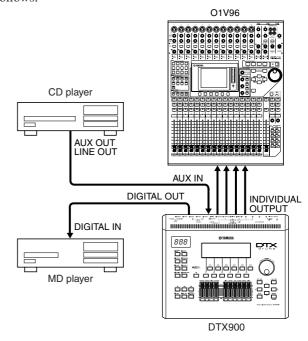
The OUTPUT (L/MONO and R) and INDIVIDUAL OUT-PUT (1 to 6) jacks produce line level audio signals regardless of whether headphones are connected or not. These jacks are mono phone type. To make audio connections via these jacks, use cables with a mono phone plug for the DTX900 and an appropriate plug for the other device.
