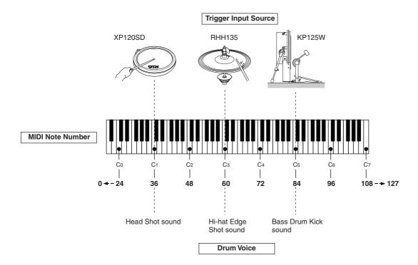
In the examples above, the Trigger Input Sources and Drum Voices listed below are assigned to the MIDI note numbers C1, C3 and C5 respectively.
